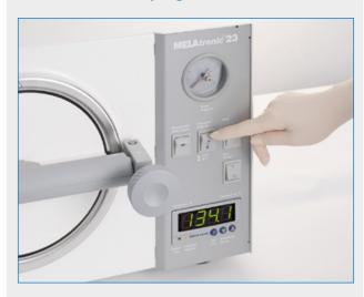
The MELA*tronic*®23 is equipped with two sterilization programs. The first program generates 134 °C / 2.1 bar for quick instrument drying. The second enables the sterilization of temperature-labile materials in a material-sensitive fashion with 121 °C / 1 bar.
